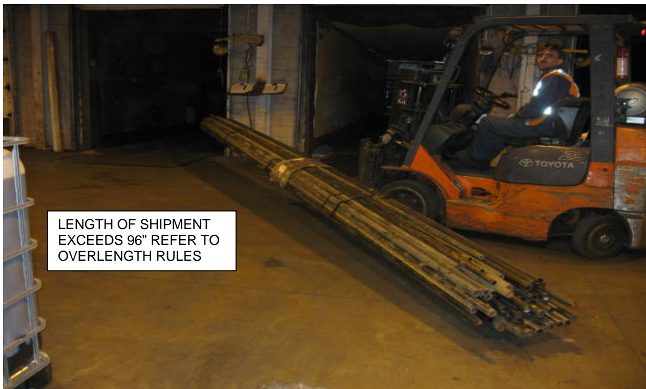
Actual shipment dimensions: 104L x 12W x 12H refer to overlength rules in Reference Guide to determine exact cube
