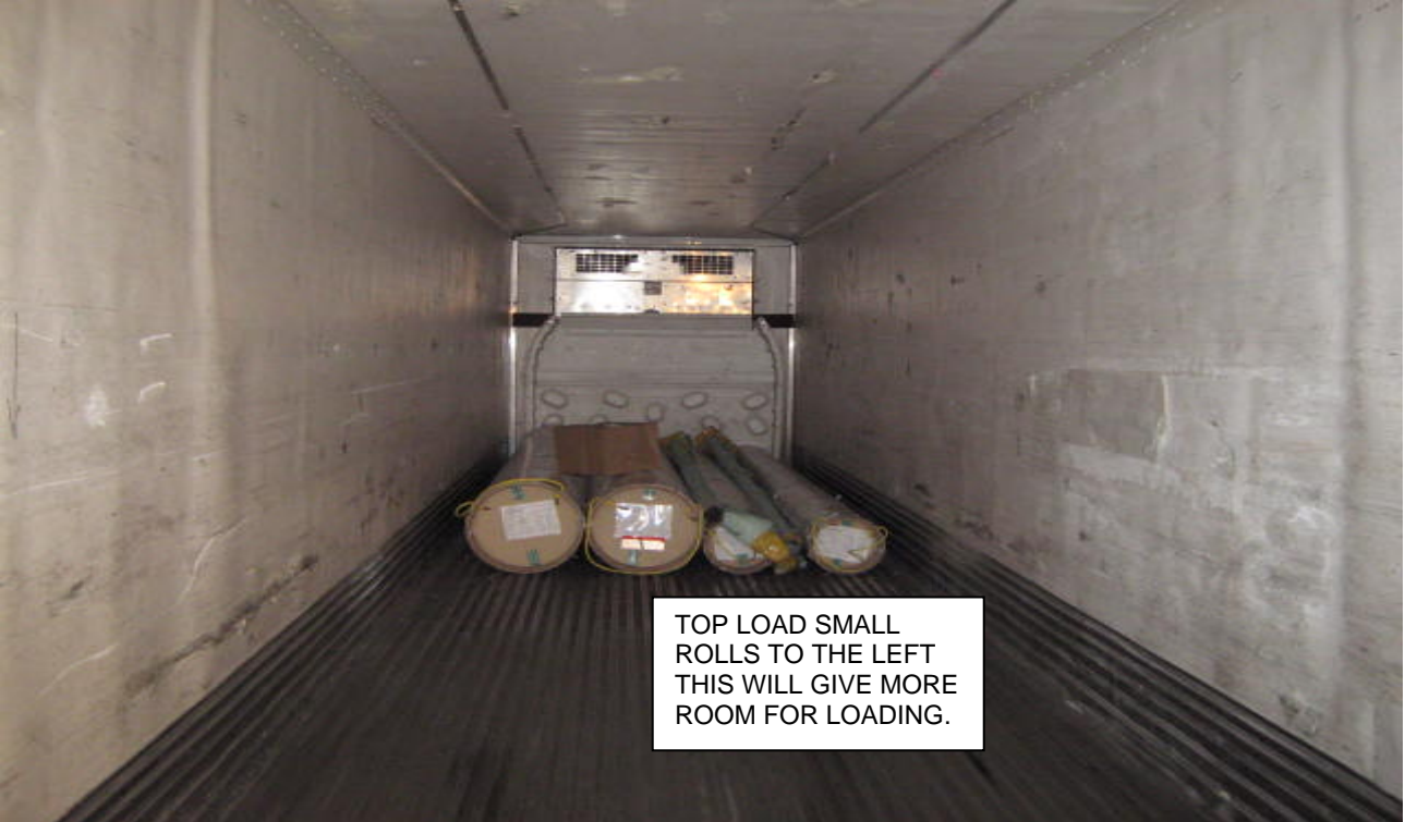
Actual dimensions are 12' feet long. Once small roles are top loaded to the left, palletized freight can be loaded on right hand side. Cube as 144L x 48W x 96H
